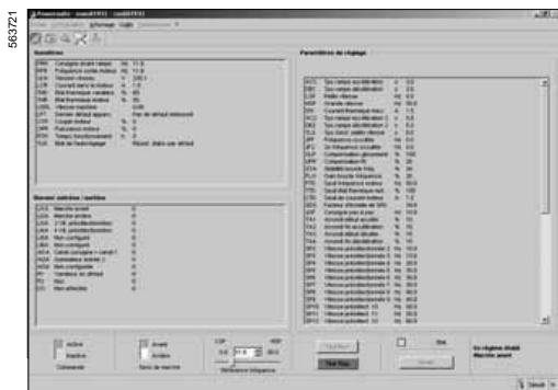
Monitoring the different parameters with PowerSuite for PC
